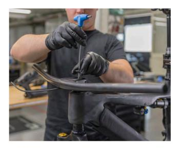
Step 2. Tighten the stem top cap with 4 mm hex key to 5 Nm of torque making sure that fork is sitting at the correct position.
