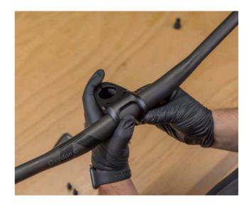
Step 1. Correctly place the handlebars in the stem slot and make sure to secure them from moving by applying the pressure to the stem clamp.
