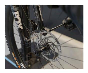
Step 3. Install the wheel and insert the axle through the fork.
