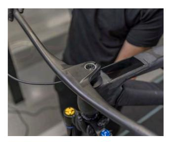
Step 1. Correctly place the handlebars in the steerer and make sure to slide it firmly all the way to the first stem spacer.
