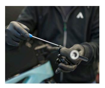
Step 3. Screw the top bolt first using a torque tool with a 4mm hex key at 4Nm.
