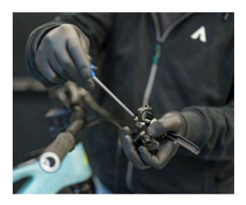
Step 1. Unscrew the brake clamp from the left or right brake lever using a 4mm hex key and place it on the handlebar to a desired position
