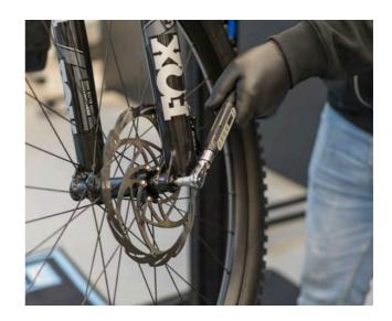
Step 4. Tighten the axle with a torque tool and a 6mm hex key using the manufactures torque indicated on the axle.
