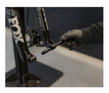
Step 2. Unscrew the front axle from the fork in order to be able to install the wheel on it.
