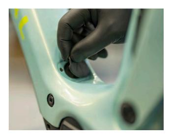
2. Slightly pull and twist the plastic cover on top of the motor to uncover the charging port.
