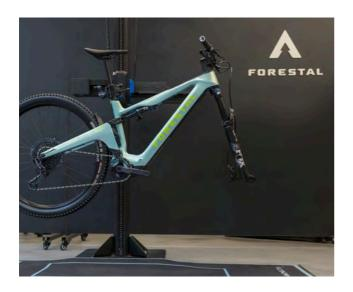
Step 1. Use a bicycle mount or lift the bicycle to install the wheel on the fork.
