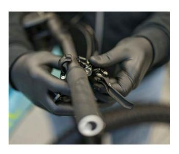
Step 2. Install the lever clamp on the brake lever.
