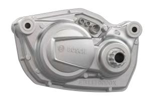
Performance line SX motor range is BOSCH electric motor unit with 250 W of power and 55 Nm of torque. It's most efficient at a cadence range of 80-100 rpm. It is IP67 graded which means it can be submerged at a depth of 1 m in water for 30 minutes. It uses the standard ISIS axle with a direct mount or standard 104 BCD chainring compatibility.
