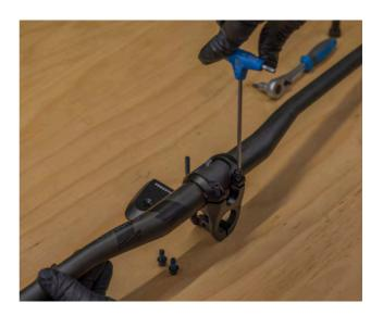
Step 3. Add two 4 mm hex bolts to the front of the stem clamp and tight it to 6 Nm.
