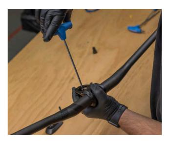
Step 2. Tighten the T25 bolts on top of the stem clamp to 6 Nm.
